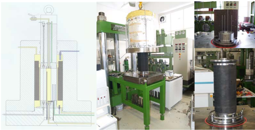
Figure 7: Laboratory investigations of thermo mechanical coupled loadings
